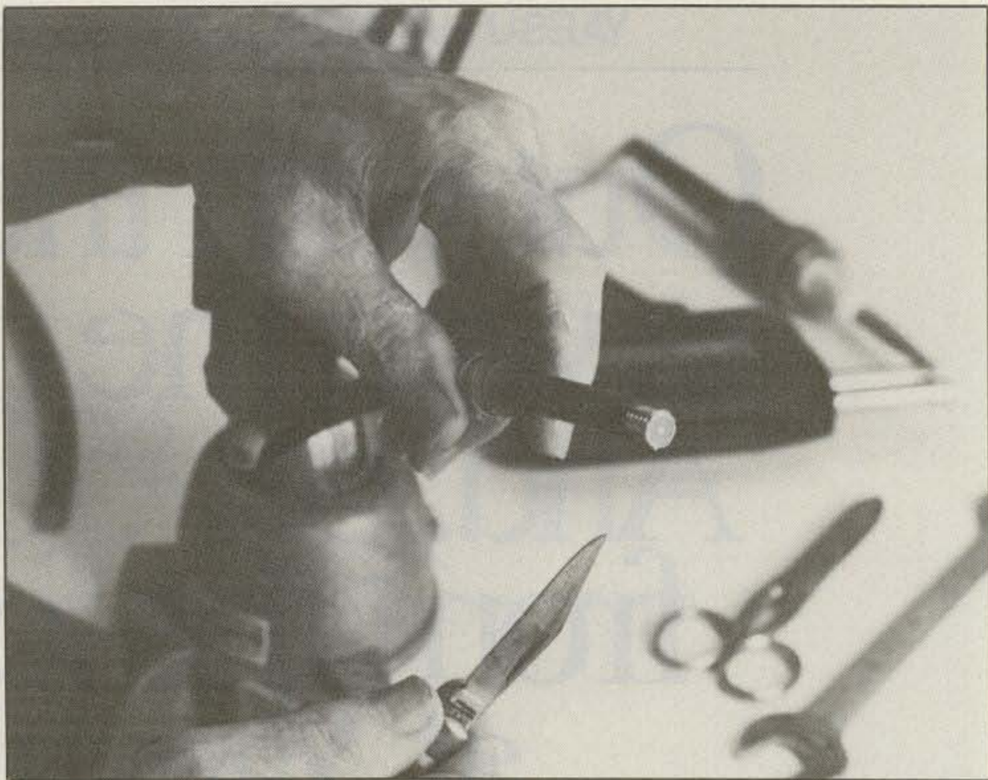
Photo 2- Remove outer jacket: After square cutting the end, slide clamp jam nut and gasket on; make a clean circumferential single cut to the shield, \frac{23}{64} inch from squared off end of the cable. Try to avoid nicking the braid.
