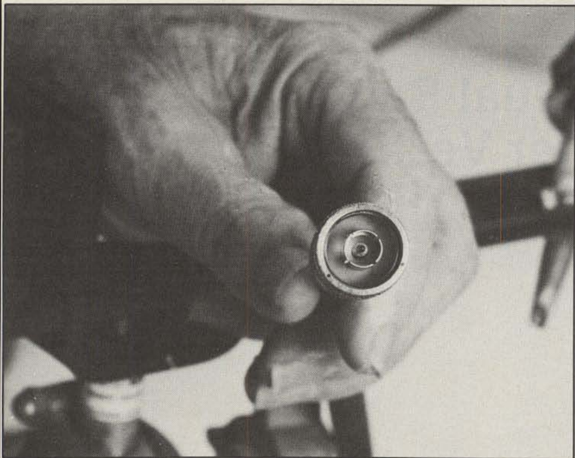
Photo 9— The pin should be centered and just scratch with your thumb as you move it over the tip of the connector.
